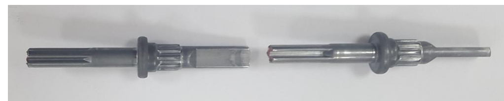
SWCH45F 11.42mm (Gear shaft)
