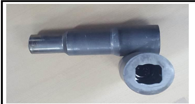
SWCH45F 34.20mm (Output shaft)
