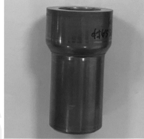
SCR420HB 38.00mm (Gear Ass'y-Sun, MID)
